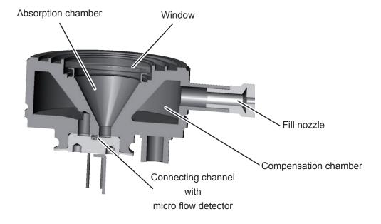
Fig. 3-2: Gas detector design principle
